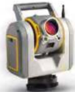
Figure 1 - Trimble SX10 Total Station
