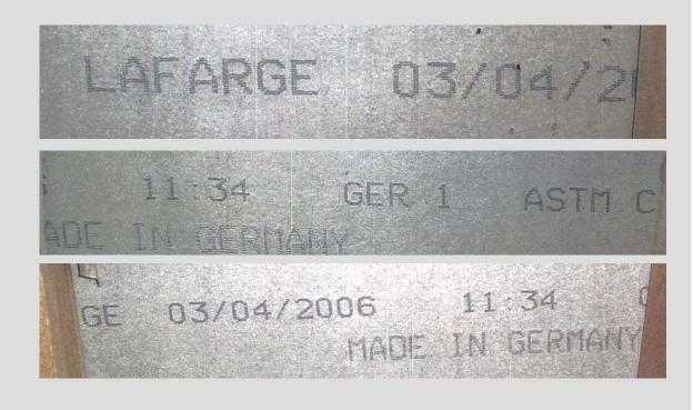
Marking: LAFARGE [DATE] [TIME] GER 1 ASTM C36
